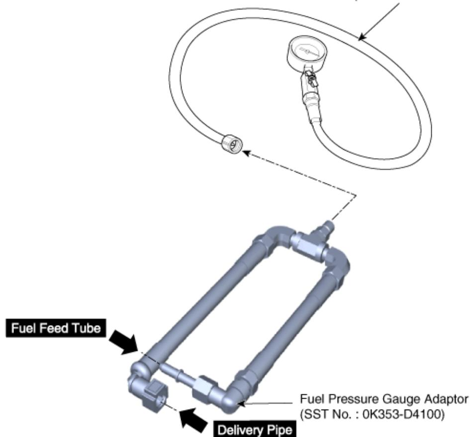
3. Inspect fuel leakage on connections among the fuel feed tube, the delivery pipe, and the SST components with ignition "ON".
